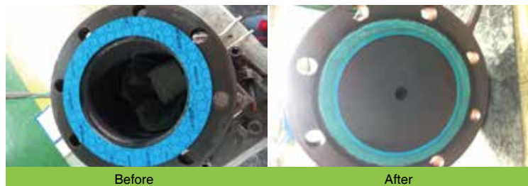
Condition: Seating Stress 120MPa and 200°C Test Result : No Adhesion
